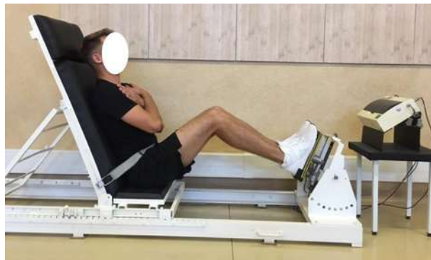
Figure 7. Global force of lower limb extensors measurement in a sitting position. The methodology described by Podgórski et al. 36 https://creativecommons.org/publicdomain/zero/1.0/deed.en .
